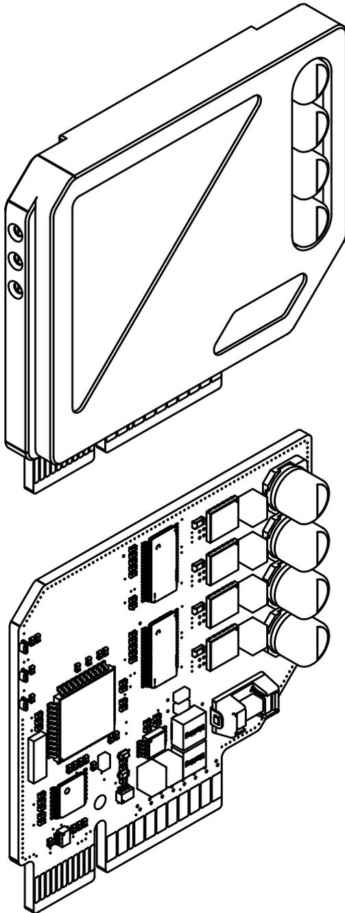
The M2 is a two-channel stepper motor driver, capable of driving small motors for laboratory automation. It offers up precision, with up to 256 microsteps per full step, power, with up to 1.3 A of maximum current per motor winding, and speed, with up to 6.2 kilosteps per second.
